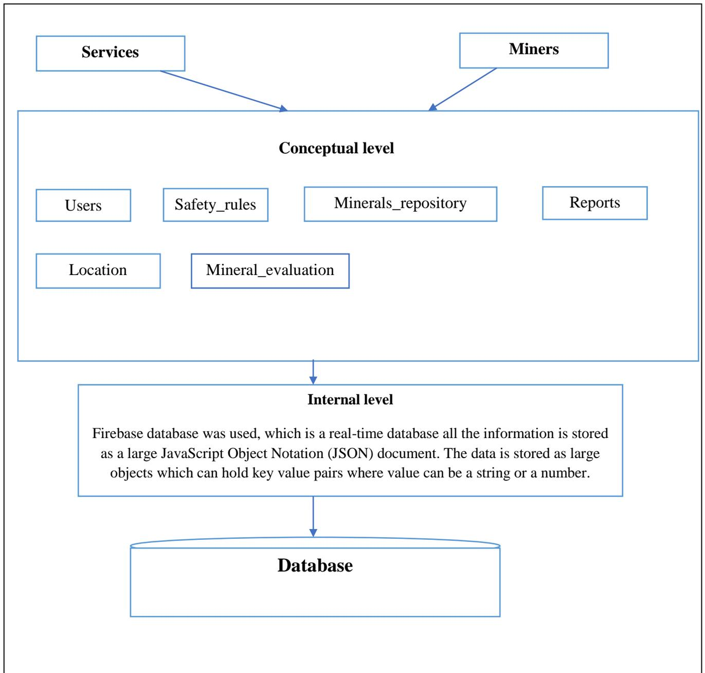
**Figure 4.5 System database architecture**
