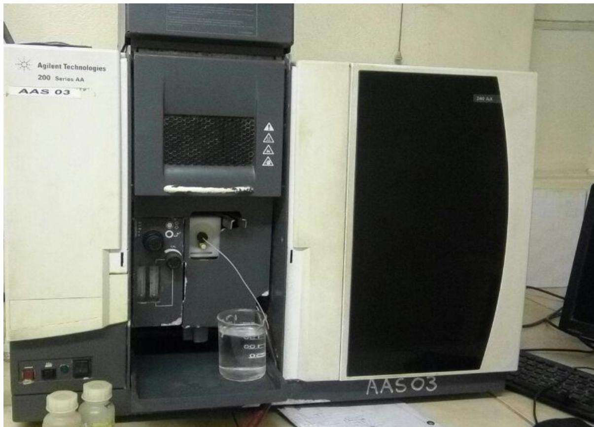
Fig 3.4: Atomic Absorption Spectrophotometer
