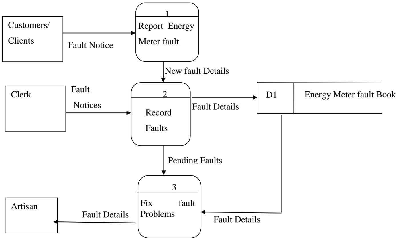
**Fig 3.3: Data Flow Diagram of the Current System**
