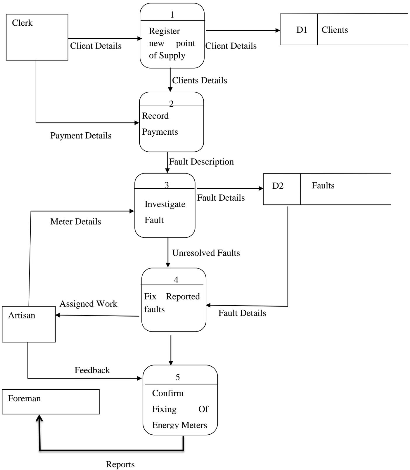
**Fig 4.3: Data Flow Diagram of the Proposed**
