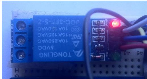
**Figure 4. 26: Diagram showing relay state after extreme temperatures were detected.**
