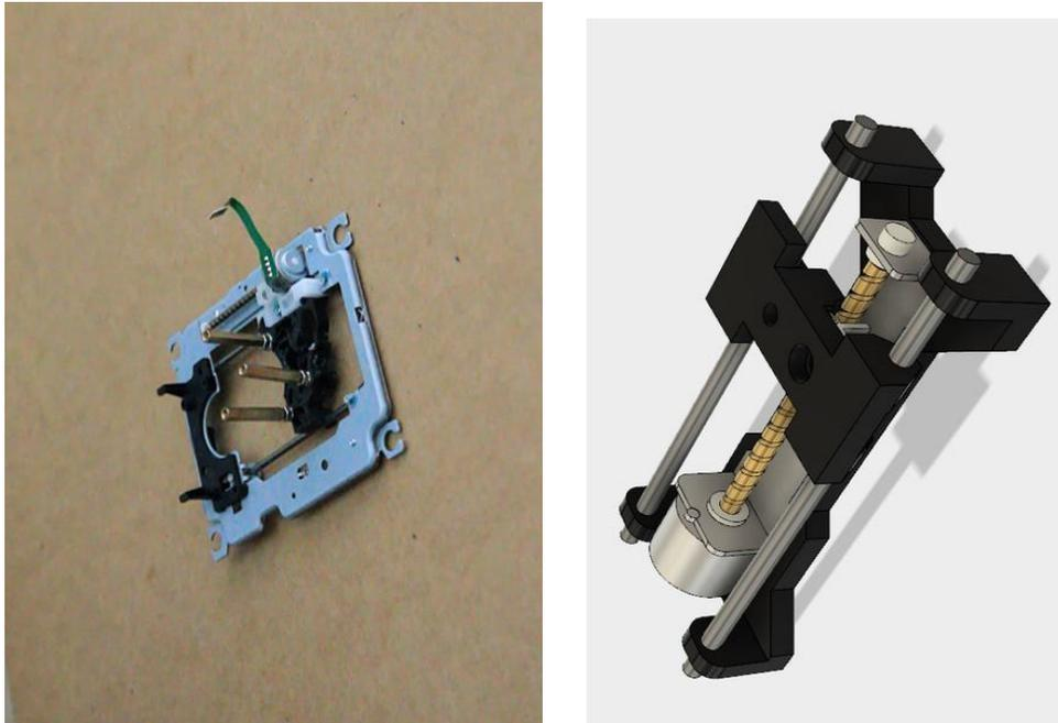
*Figure 2.26 Bipolar Stepper Motor (CD-ROM)*
