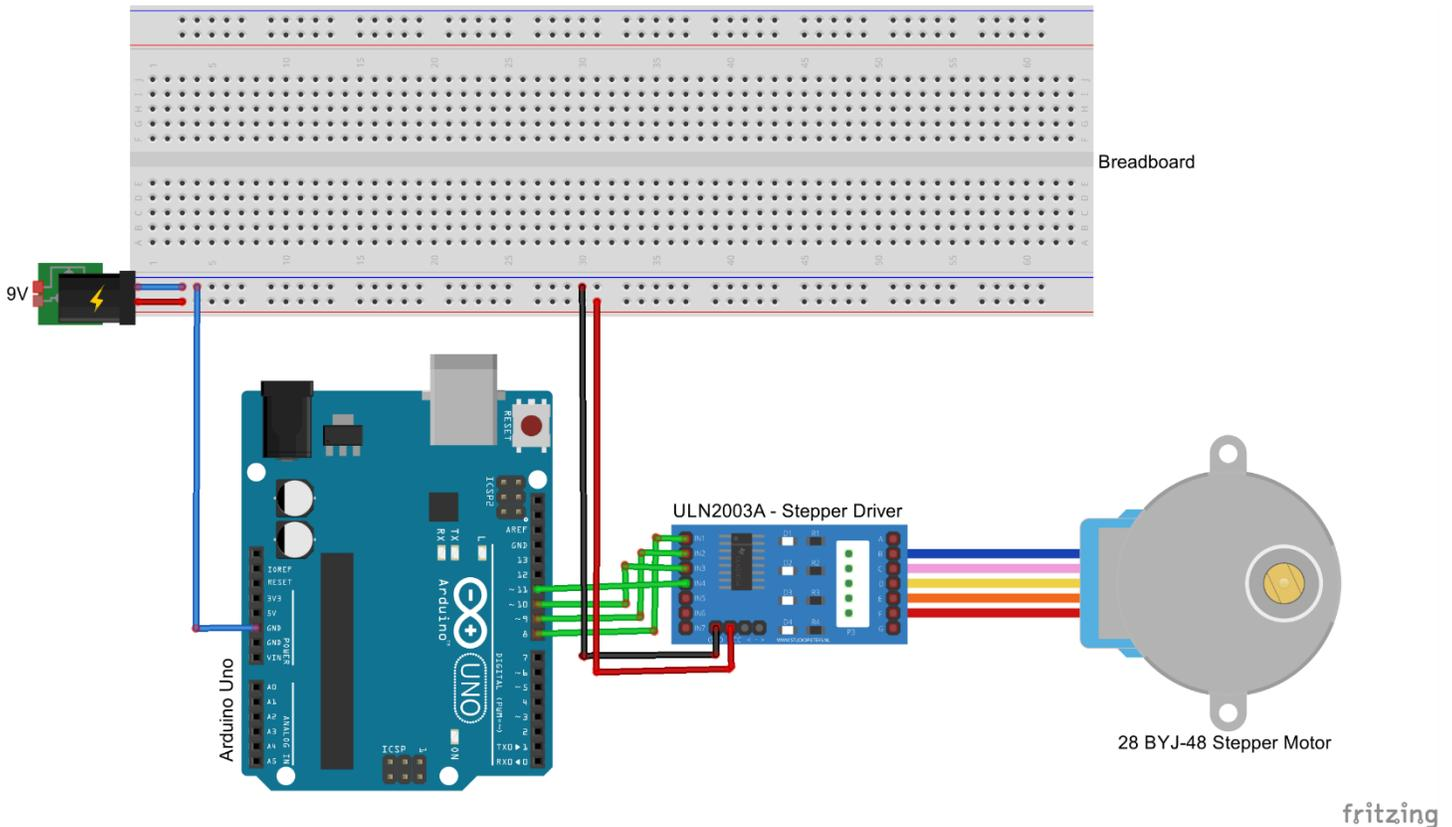
*Figure 3.3 Arduino to ULN2003A Unipolar Stepper Motor Driver Connection (Fritzing Circuit)*
