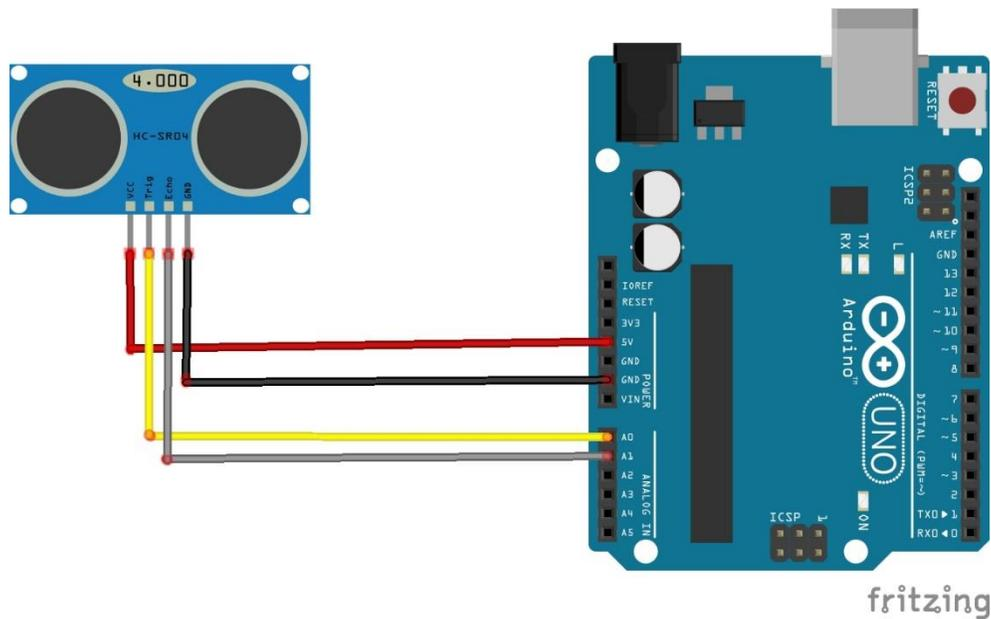
Figure 3.4 Arduino Uno to Ping Ultrasonic Sensor Connection (Fritzing Circuit)
