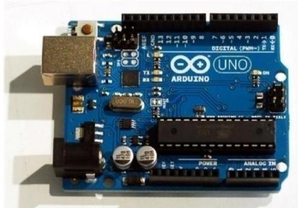
Figure 2.22 Arduino Uno Microcontroller
