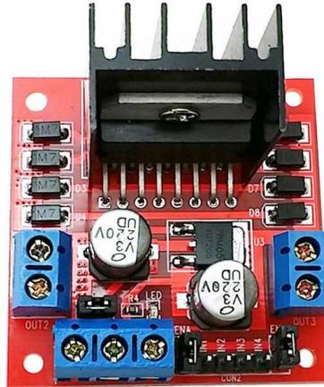
Figure 2.25 Bipolar Stepper Driver L298N
