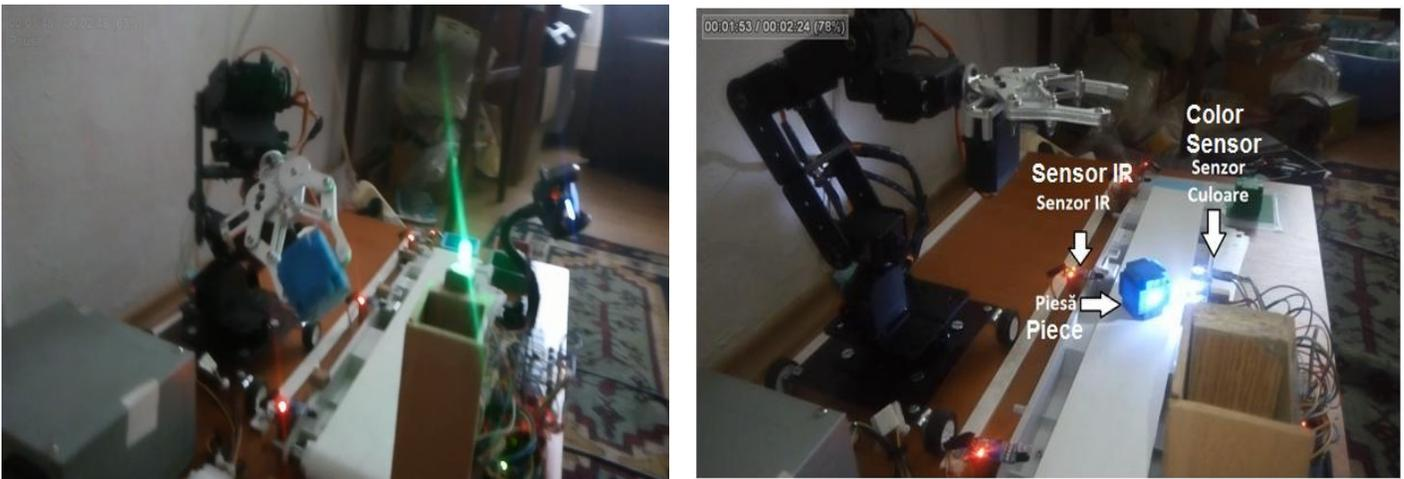
Figure 2.17 Robotic arm grabs objects from the conveyor belt
