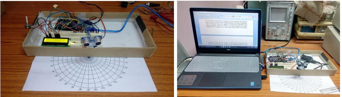
*Figure 2.16 Prototype: Ultrasonic distance meter*
