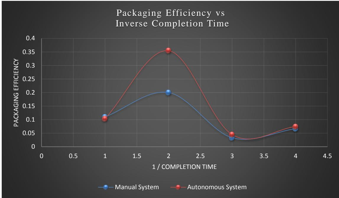
Figure 4.13 Variation of Efficiency With Inverse Completion Time
