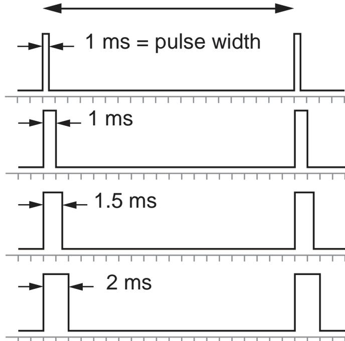
Figure 2.28 SG90 Servo Control Signal Pulse Train
