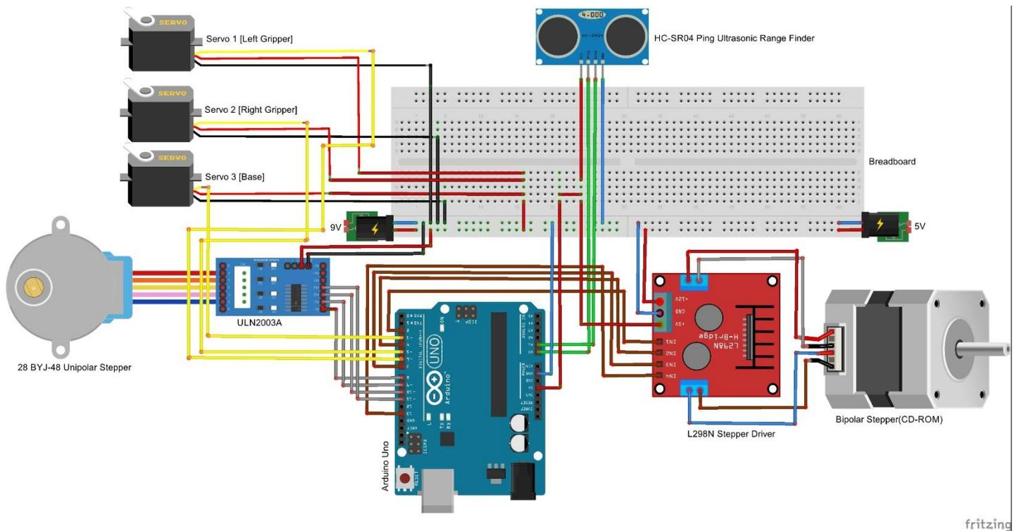
Figure 3.7 Overall System Schematic (Fritzing Simulation)
