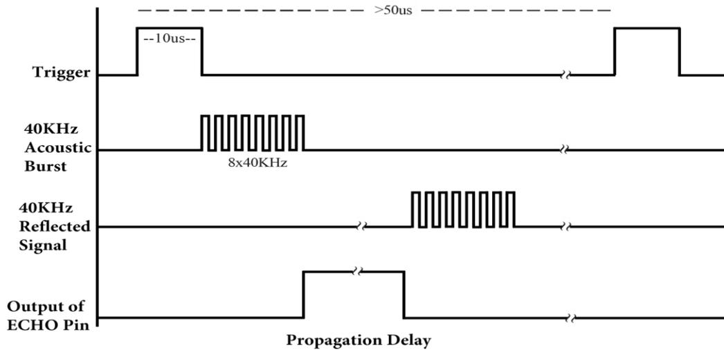
Figure 2.9 HC-SR04 Module Timing
