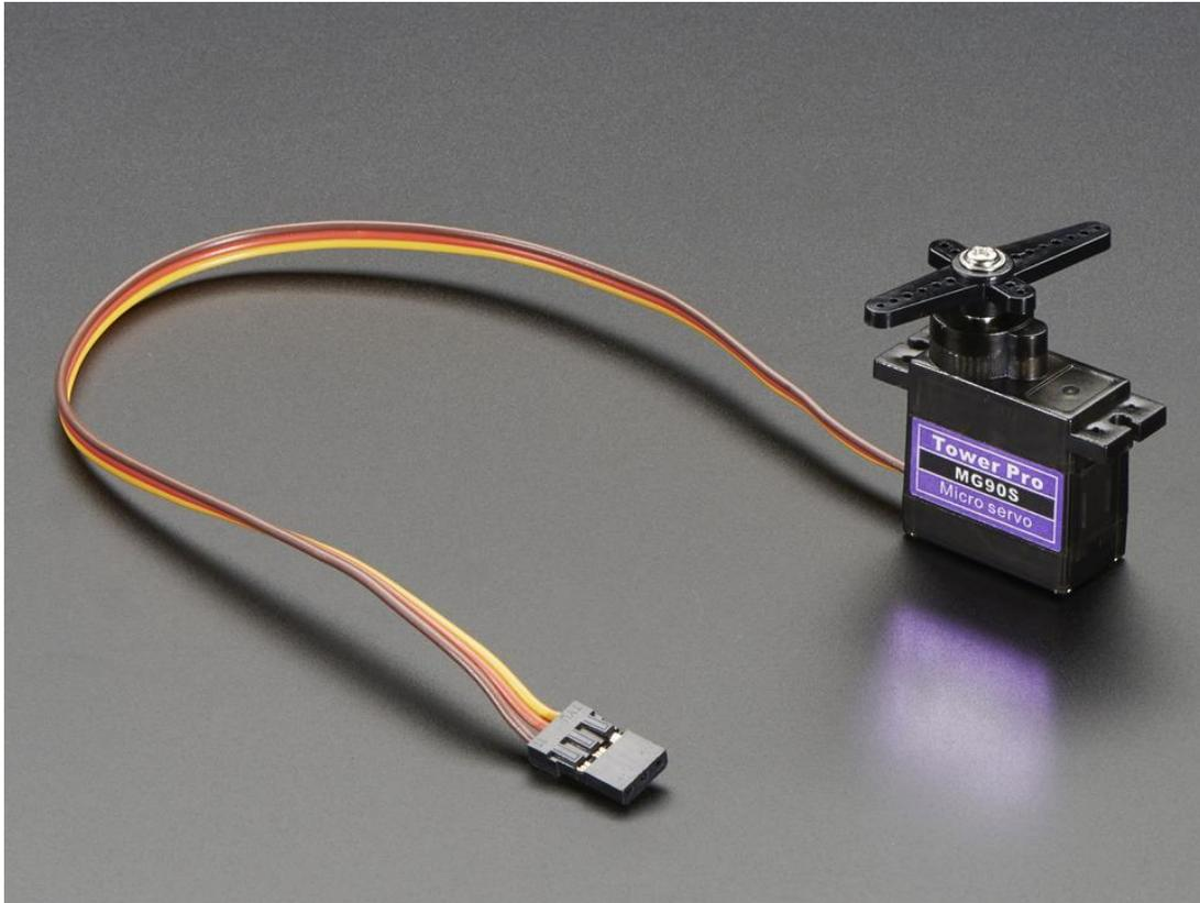
Figure 2.30 Micro Servo (MG90S High Torque Metal Gear)
