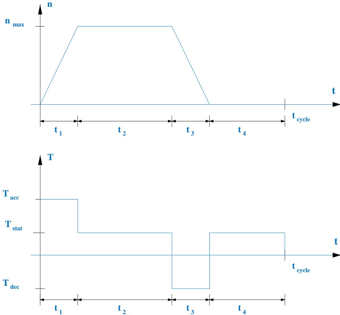
Figure 4.14 Cycle for an industrial robot servo motor.
