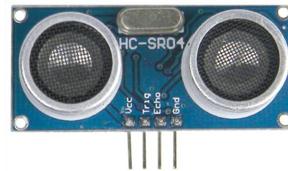
Figure 2.29 The HC-SR04 Ultrasonic Module
