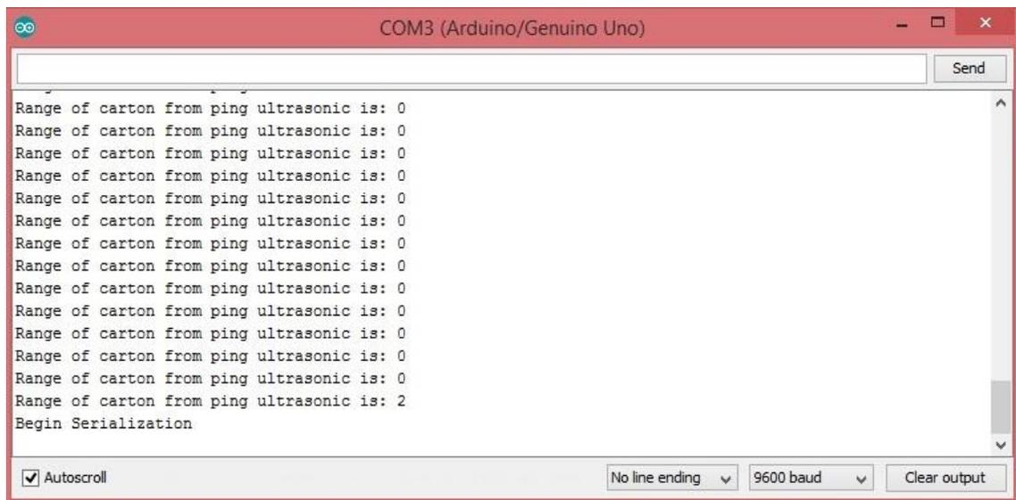
Figure 4.7 Image Capture: Carton Detected, Begin Serialization
