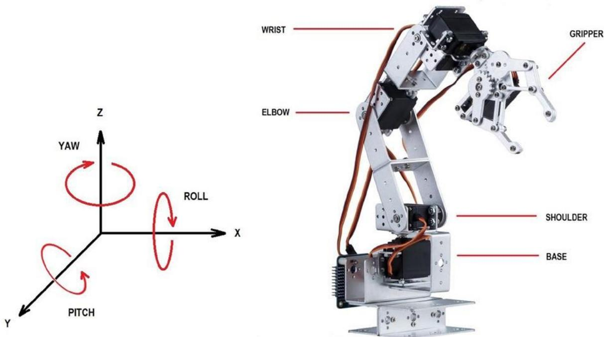
Figure 2.13 3D space depiction of roll, yaw, and pitch in a robotic arm
