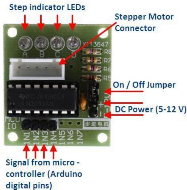
Figure 2.24 Unipolar Stepper Driver ULN 2003A
