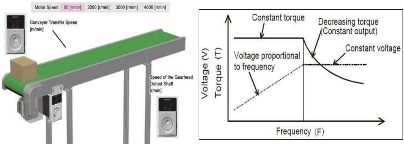
Figure 2.6 Characteristic Curve of Conveyor Load Variation with Motor Velocity
