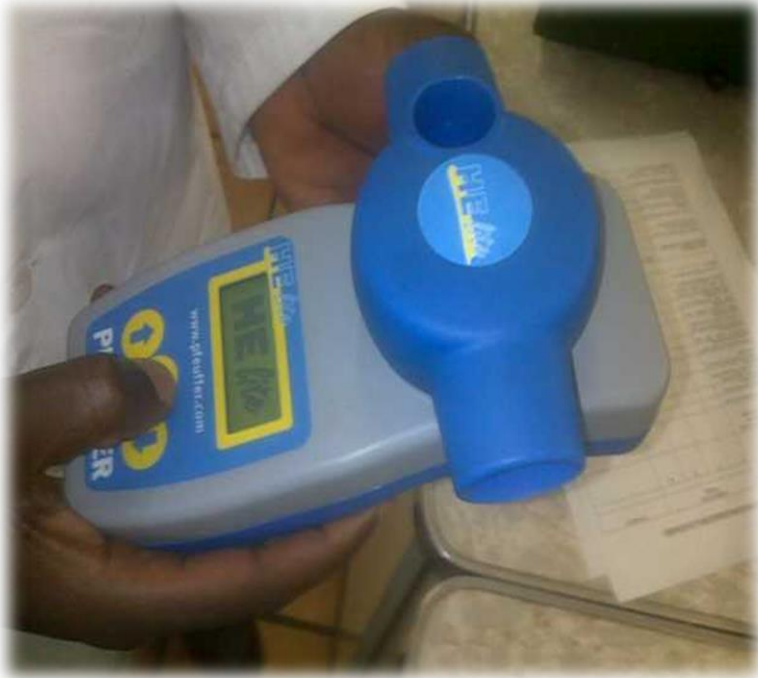
Picture 4: Pfeuffer Moisture determination meter used by the researcher.
