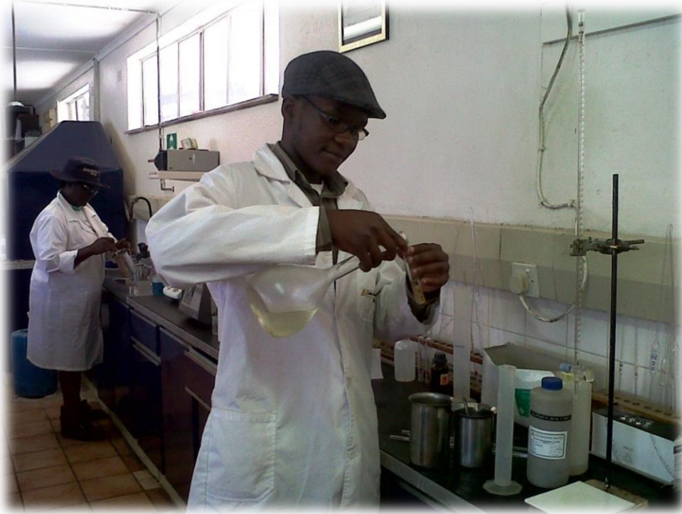
Picture 3: The researcher adding tetrazolium solution to a sample during the determination of germination capacity.
