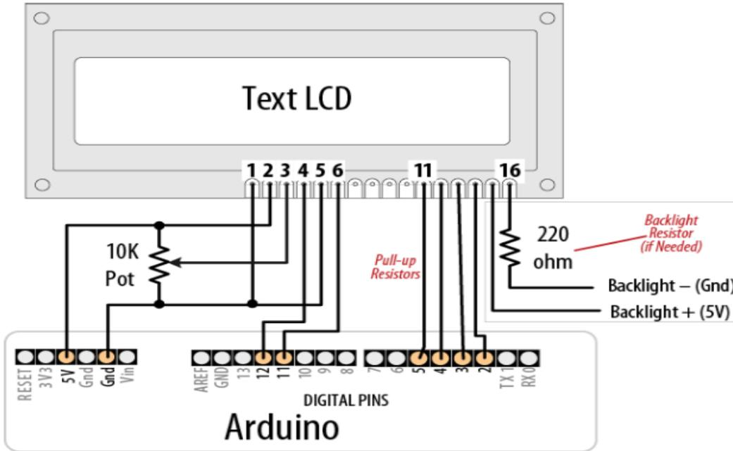
Fig 3.7 : connections for LCD
