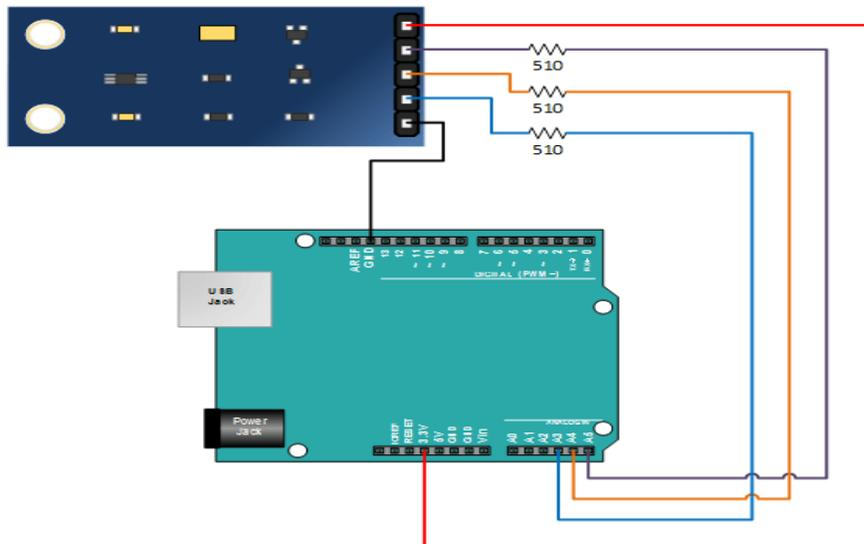
Fig 3.6: BH1750 connection with arduino
