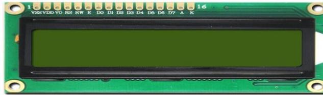
Fig 2.2: Liquid crystal display
