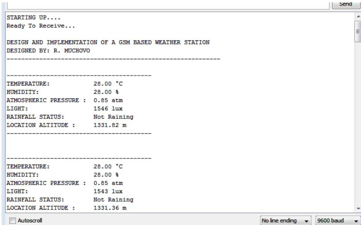
Figure 4.4: overall system measurements
