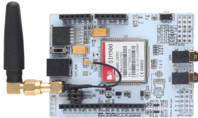
Fig 2.4: Arduino sim900 gprs/gsm shield
