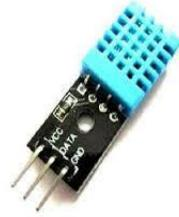
Fig 2.5:DHT11 humidity and temperature sensor
