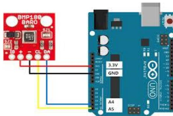
Fig 3.3: BMEP280 connection with arduino
