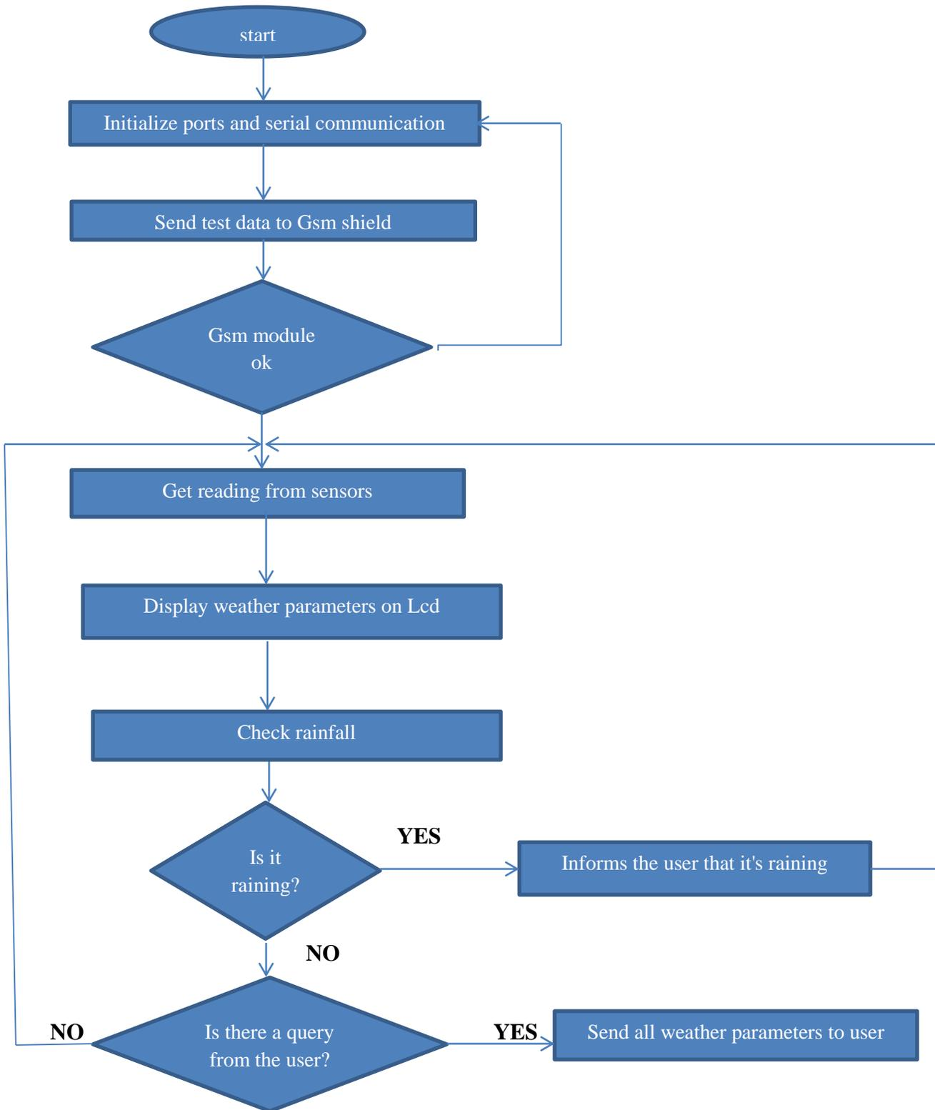
Fig 3.8: system flowchart diagram
