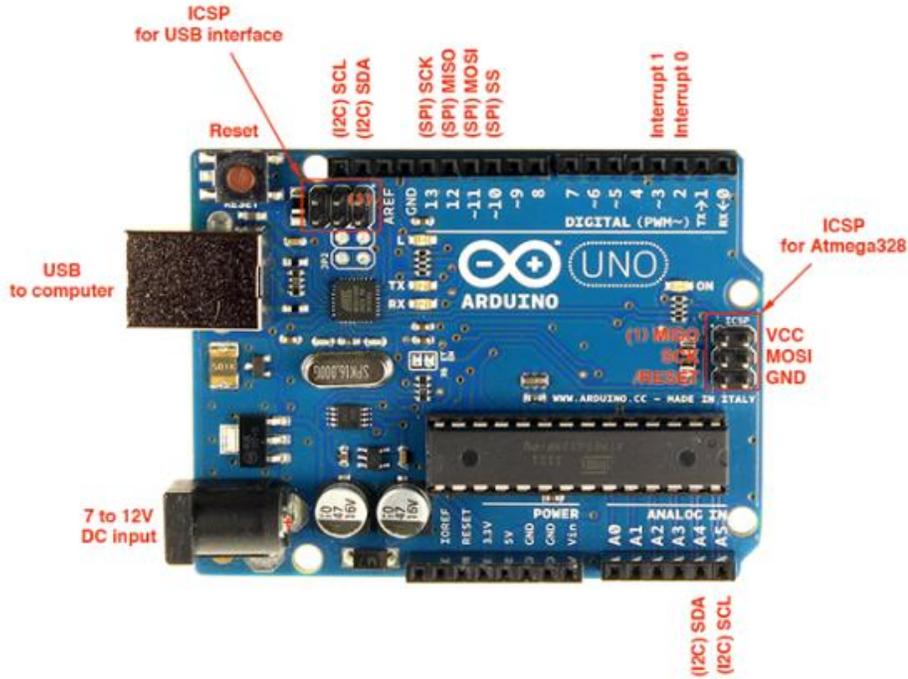
Fig 2.3: Arduino micro-controller board
