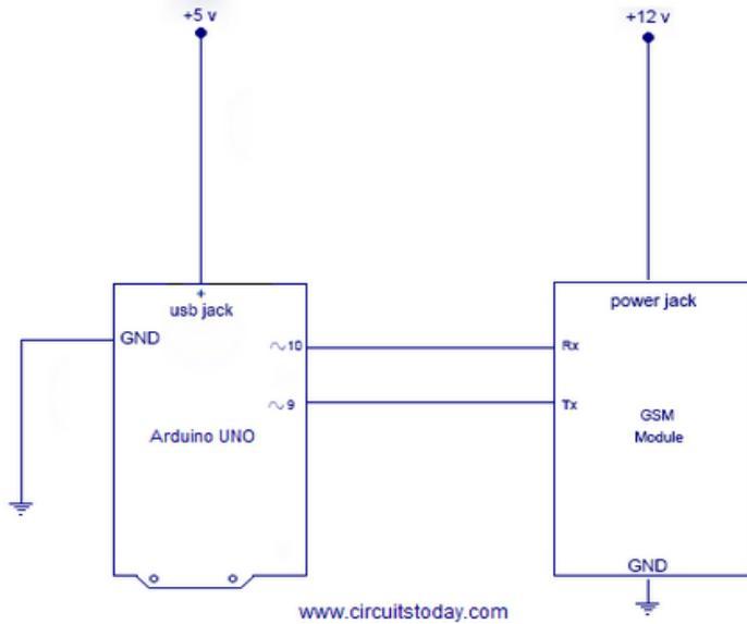
Figure 3.5: Gsm shield to arduino connection
