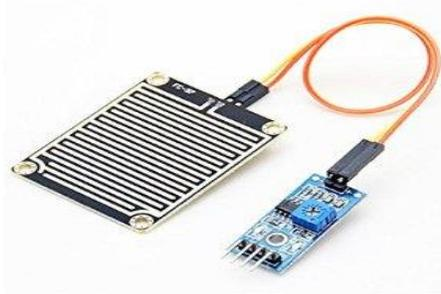
Fig 2.7: raindrop detection sensor
