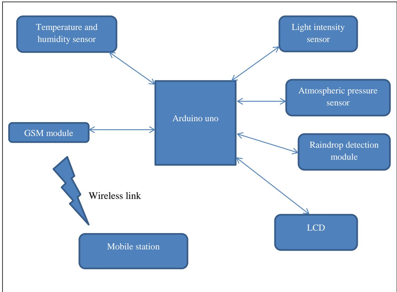
Fig 3.1: system block diagram
