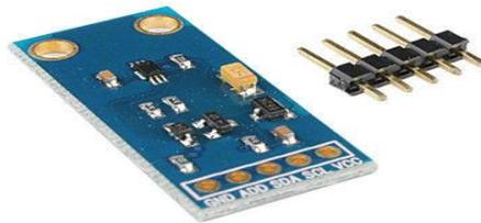
Fig 2.8 : BH1750 digital light sensor
