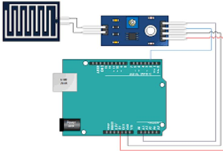
Figure 3.4: rain sensor module to arduino connection
