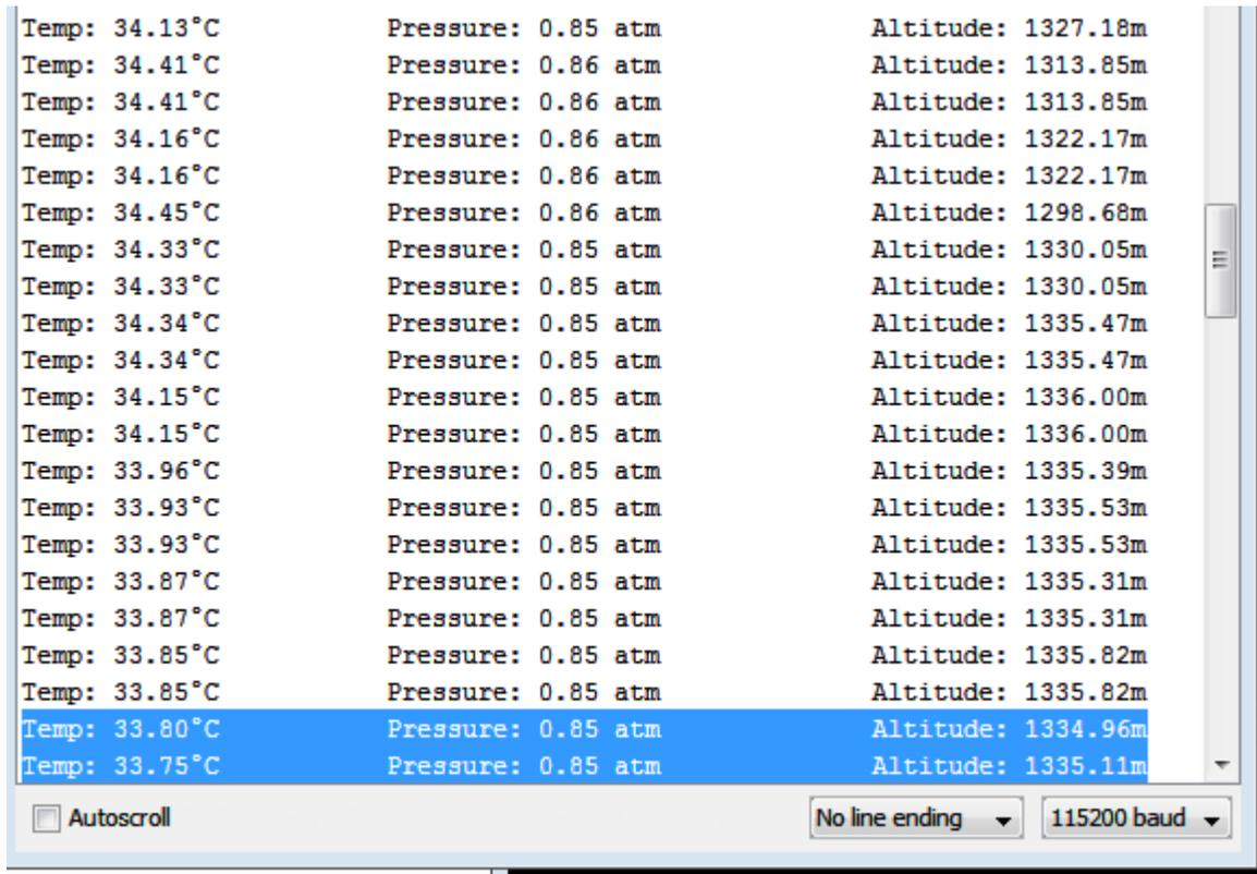
Figure 4.3: BMEP280 pressure, altitude and temperature measurements
