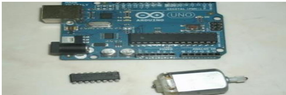
Fig 2.6: A dc motor with an Arduino Uno and a L293D photograph [16].
