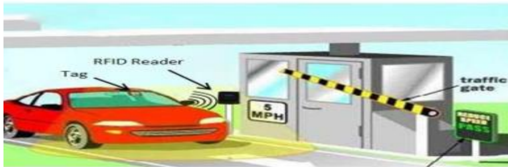
Fig 3.2 Interactions between RFID reader and vehicle tag [2]
