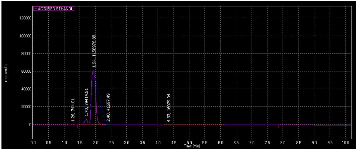
Fig. C4: HPLC chromatogram with calculated area for acidified ethanol.
