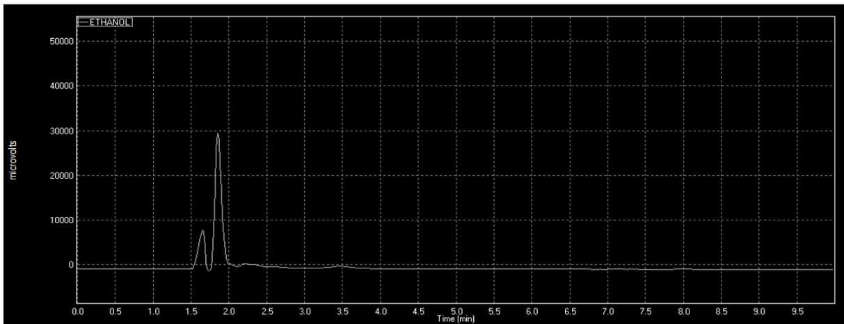
**Fig. C11:** HPLC chromatogram for ethanol.
