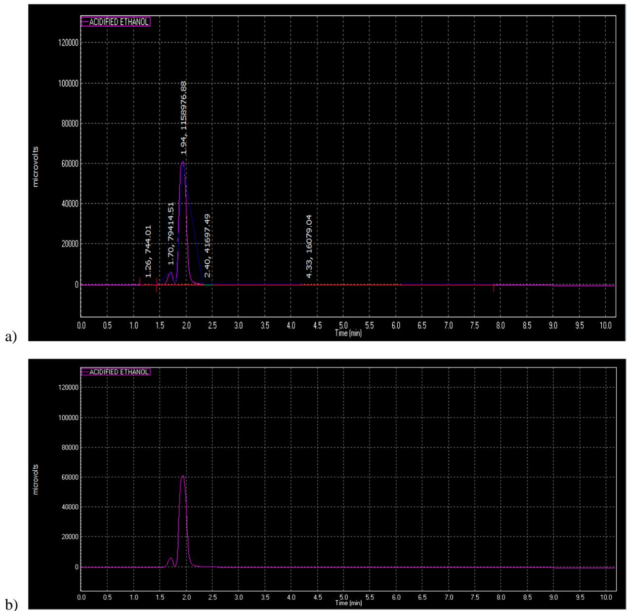
**Fig 4.1:** HPLC chromatograms (a) with calculated peak area and (b) without area of acidified ethanolic extract.
