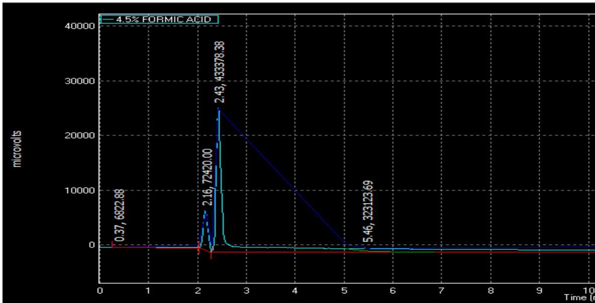
**Fig. C2:** HPLC chromatogram with calculated area for 4.5 % formic acid in water.
