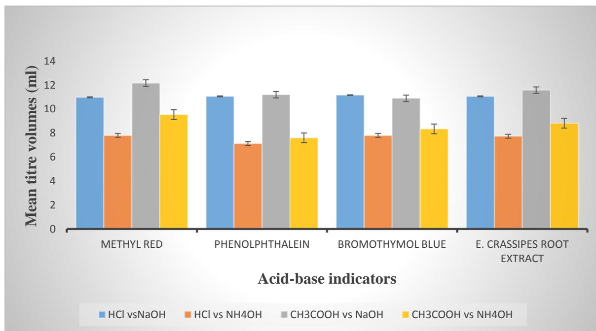
**Fig. 4.7:** Mean titre volumes obtained during four titration processes, HCl-NaOH, HCl-NH<sub>4</sub>OH, CH<sub>3</sub>COOH-NaOH and CH<sub>3</sub>COOH-NH<sub>4</sub>OH.
