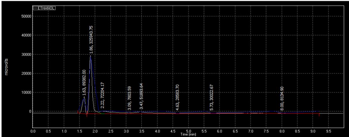
**Fig. C10:** HPLC chromatogram with calculated area for ethanol.
