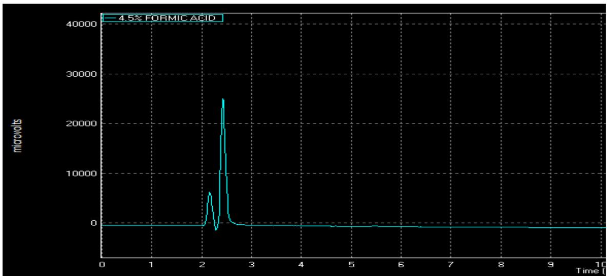
**Fig. C3:** HPLC chromatogram for 4.5 % formic acid in water.
