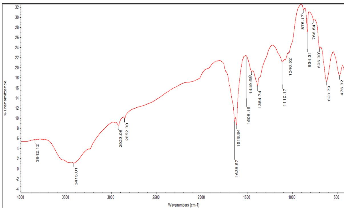
**Fig. 4.6:** FTIR results of *E. crassipes* root extract (0.1 % HCl in ethanol extract) vibrational frequencies.
