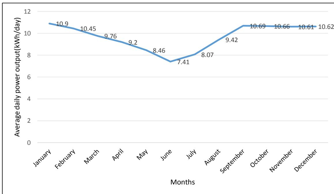
**Fig 4.4 Average daily power output per month from an array of 2.115kW.**
