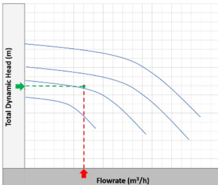
**Fig 2.6 an example of solar pump chart for determining energy demand.**
